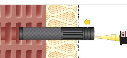
5. Press ResiTHERM® 37 onto mixing nozzle and push it carefully into the drill hole
