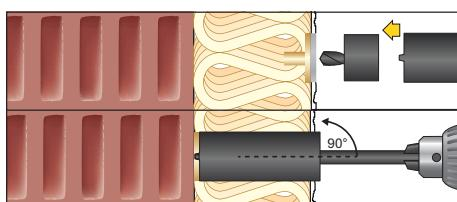
1. Put drilling aid on core bit; drill with cordless screwdriver (without impact) through the insulation material up to the hollow brick wall (remove drilling aid after the first 10 mm)
