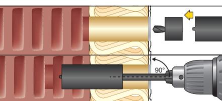
3. Put drilling aid on core bit and drill min. 130 mm into the hollow brick wall (remove drilling aid after the first 10 mm)
