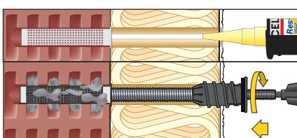
7. Fill the plastic sleeve completely with composite mortar (start from the beginning). For number of strokes see mounting instructions at [www.celofixings.com](http://www.celofixings.com)
