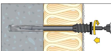
6. Screw in the ResiTHERM® 16 with the hexagon bit (included) and a cordless screwdriver until the seal is pressed against the plaster.
