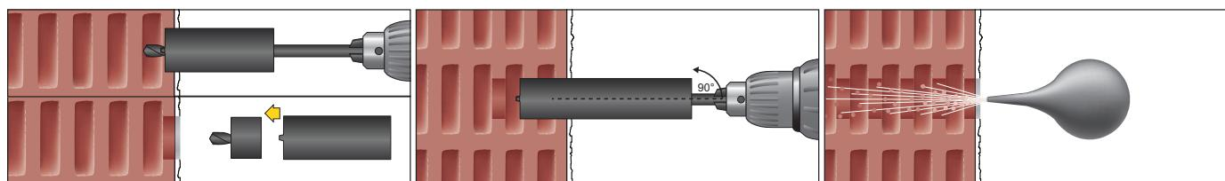
1. Put drilling aid on core bit; drill with cordless screwdriver (without impact) into the hollow brick wall; remove drilling aid after the first 10 mm)
