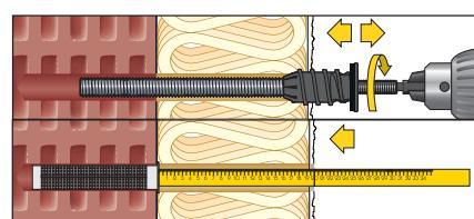
4. Enlarge the opening in the plaster for the collar of the plastic sleeve to 26 mm. To do this, briefly screw the thermal separation module in and out through the plaster for only approx. 2 thread turns or ream the plaster with a drill or drill with a bigger 26 mm drill.
