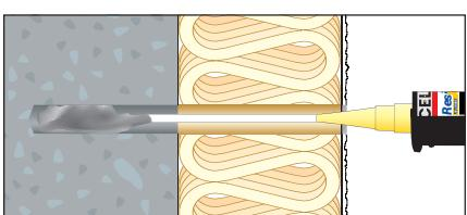
5. Fill at least 2/3 of the drill hole with composite mortar (start from the beginning). For number of strokes see mounting instructions at [www.celofixings.com](http://www.celofixings.com).
