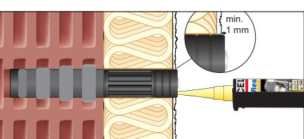
6. Fill ResiTHERM® 37 with injection system ResiFIX; the end of the filling process can be clearly felt
