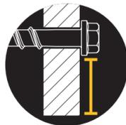
**Expansion-free anchoring** allows low edge distances and spacing
