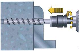
3. Install the anchor with a torque wrench or an Impact Screw Driver
